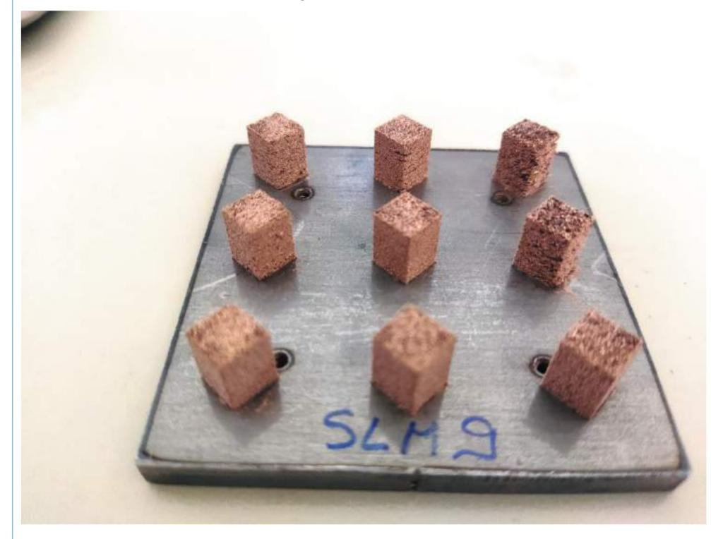
Realization of lattice structures is in progress
