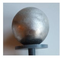
Now they are prototyping some tools for internal use, this one: it's a part of a checking tool designed for testing electric equipment to compliance with the standard "IEC 60529:1989+A1:1999+A2:2013 Applies the to classification of degrees of protection provided by enclosures for electrical equipment with a rated voltage not exceeding 72,5 kV"
